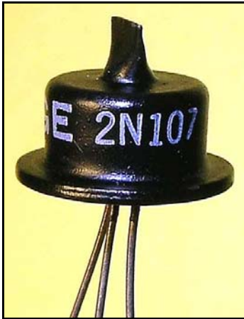
Transistor Size (7/8" OD X 3/8") Date Code 5-39 (1955 Week 39) on Back
