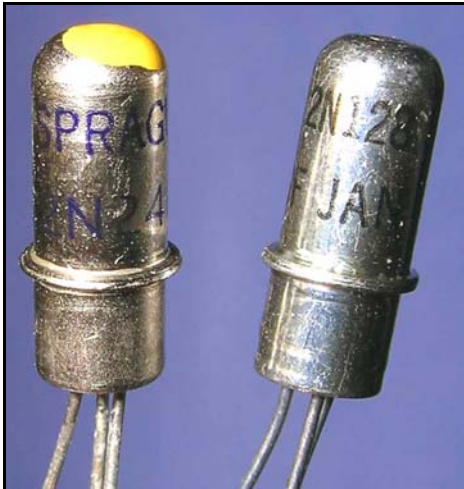
Transistor Size (1/8" OD X 3/8") Standard TO-24 Case
